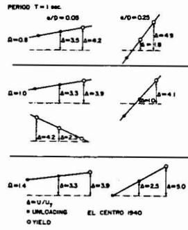
Figure 5. Position of Structure at Instant of Maximum Edge Displacement
